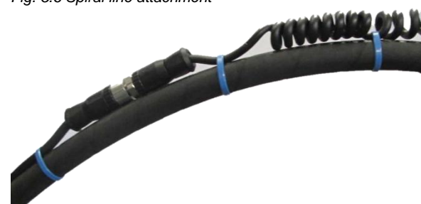
Fig. 5.6 Spiral line attachment
