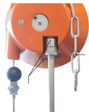
Fig. 5.5 – Fine-tuning of the spring balancer
