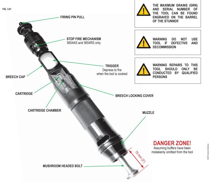
**NOTE** - every tool in the **CASH**<sup>®</sup> range is stamped with the maximum permitted (PROOF) cartridge, showing the maximum grains (GRN) that should be used.
