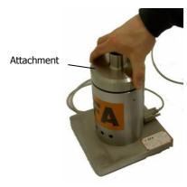
To change the sensors, first loosen the connection cable and unscrew the attachment.
