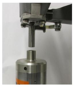
Insert the cattle stunner vertically into the guide of the attachment. Avoid tilting the cattle stunner. This is the only way to obtain a correct evaluation result.
