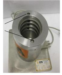
Then loosen the 4 M8 screws on the underside of the plate and remove the bracket cpl. from the plate.
