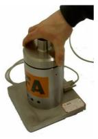
Screw on the new attachment and tighten with the mandrels. **There are no torque values specified.**
