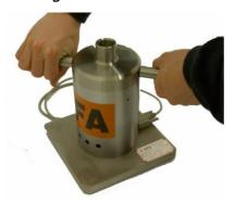
To change the attachment, insert mandrels into the opening of the bracket cpl. and unscrew the attachment.
