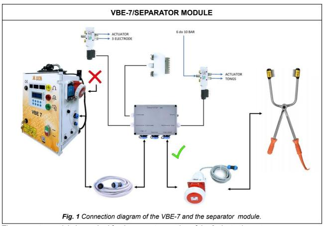
The separator module is required for the correct operation of the 3 electrode system.
