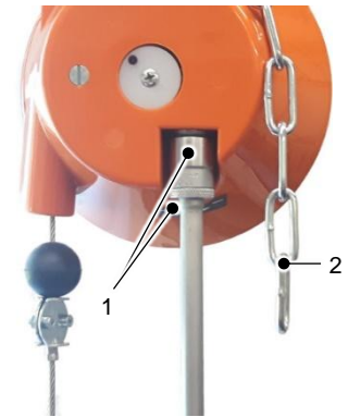
Fig. 5.2 – Fine-tuning of the spring balancer
